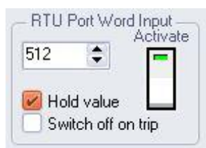
Figure 8.1.12.m: KG/KH-RTU frontend simulator Modbus-RTU word input panel.
