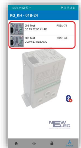
Figure 8.2.2.b: KG/KH-RTU app showing results of KG/KH-RTU relays detected.
