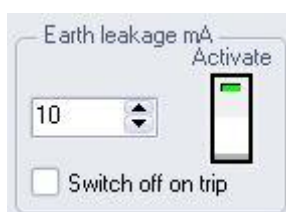
Figure 8.1.12.h: KG/KH-RTU frontend simulator earth leakage level panel.
